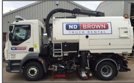
Short wheelbase and space between axles for equipment
